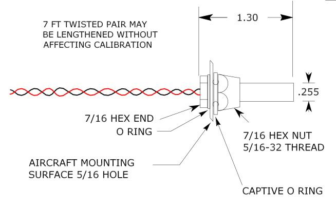
NOTES: THE TEMPERATURE SENSOR MOUNTING SHOULD BE IN A PLACE THAT IS FREE OF EXHAUST GASES OR COWL FLAPS AIRFLOW. THE IDEAL PLACE IS TWO FEET OUT FROM THE WING ROOT ON THE BOTTOM OF THE WING. SENSOR LEADS MAY BE LENGTHENED OR SHORTENED WITHOUT AFFECTING
